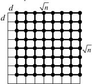
Figure 5. NoC – interconnecting n communicating modules arranged in regular mesh, size of each is d X d
