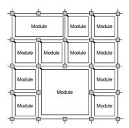
Figure 1. QNoC custom topology example - irregular mesh
