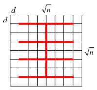
Figure 6. Non-Segmented Bus - interconnecting n communicating modules arranged in regular mesh, size of each is d X d
