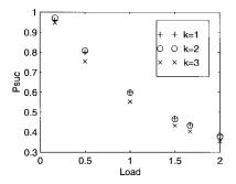
Fig. 13. The success probability per trial,  $P_{\rm suc}$ , as a function of the load for n=3 and m=2.
