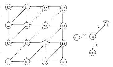
Fig. 6. A Markov chain for a system with n = 2, m = 3, and k = 2.
