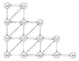
Fig. 2. A Markov chain for a system with n = 4, m = 1, and k = 2.
