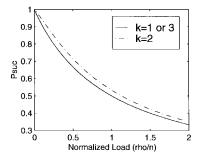
Fig. 12. The success probability per trial,  $P_{\rm suc}$ , as a function of the load for n=3 and m=1.
